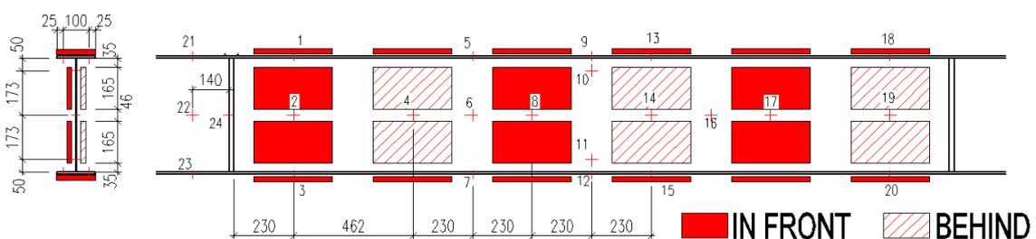
Fig. 8 Layout of flexible ceramic pads and thermocouples
