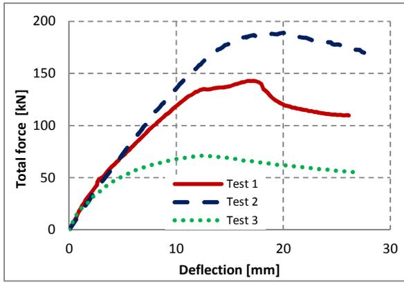
Fig. 11 Vertical deflection of bottom flange at midspan
