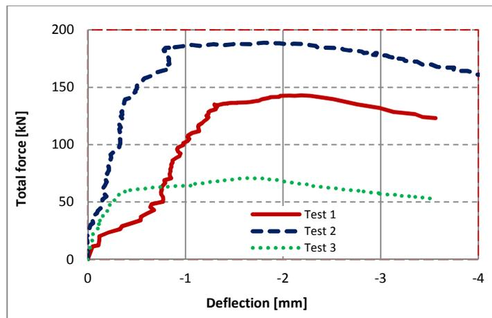
Fig. 13 Horizontal deflection of bottom flange at midspan
