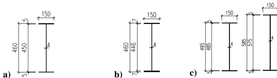
Fig. 1 Cross-section: (a) Test 1; (b) Test 2; (c) Test 3
