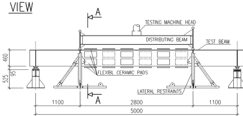
Fig. 2 Scheme of experiment
