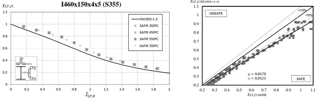
Fig. 4: Comparison between the numerical results calculated with SAFIR and LTB resistance of beams with welded class 4 cross-sections according to EN1993-1-2.
