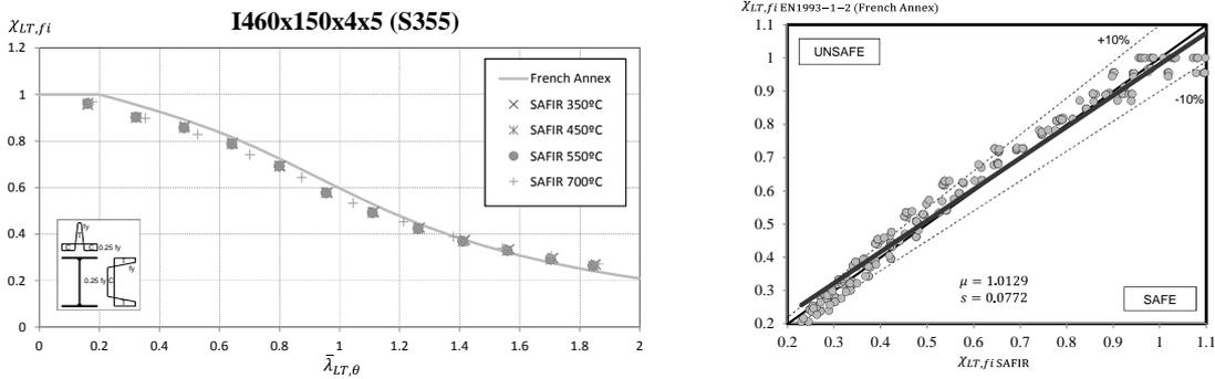
Fig. 5: Comparison between the numerical results calculated with SAFIR and LTB resistance of beams with welded class 4 cross-sections according to French National Annex of EN1993-1-2.
