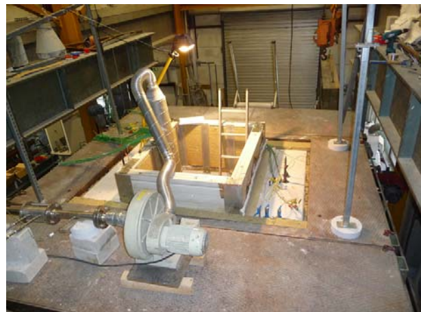
Fig. 6 Façade elements, which come through the furnace ceiling. In order to prevent an overheating in the tower a ventilator, blowing air into the lower area of the tower, guaranteed a continuous slow air draft from the tower floor to the ambient air
