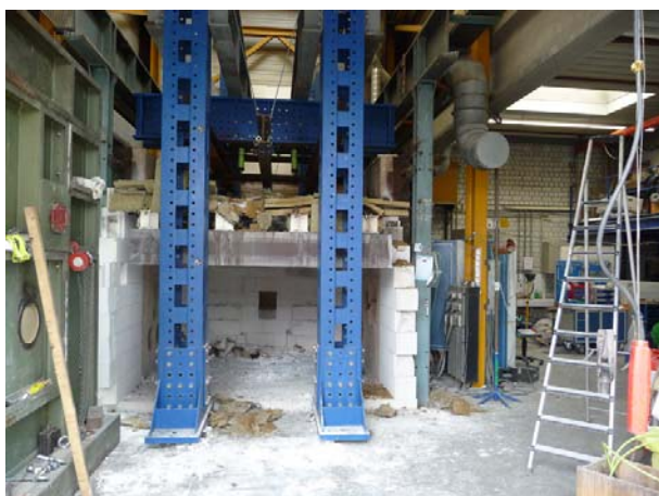
Fig. 3 View from outside; the blue and grey columns and beams are the load admission
