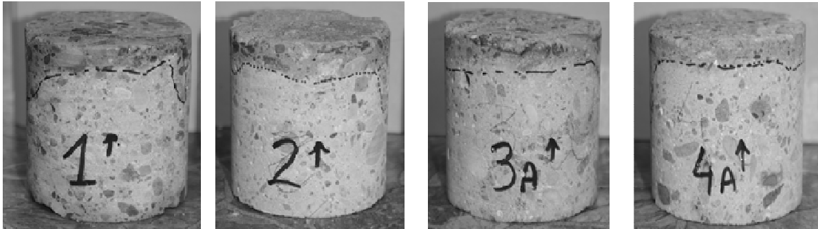
Fig. 4 Discoloration depth corresponding to the depth of destruction of the drilled concrete cores
